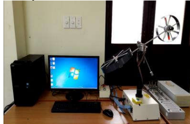
Figure 4.5: Model of TRMS experimental table
